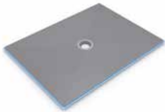
04 wedi Fundo Ligno Our newest Fundo model: Floor level 19 mm profile designed especially for suspended wood subfloors. Like all wedi shower bases it is pre sloped, and waterproof. Comes with 100 x 100 mm drain cover. Customisable on site.
